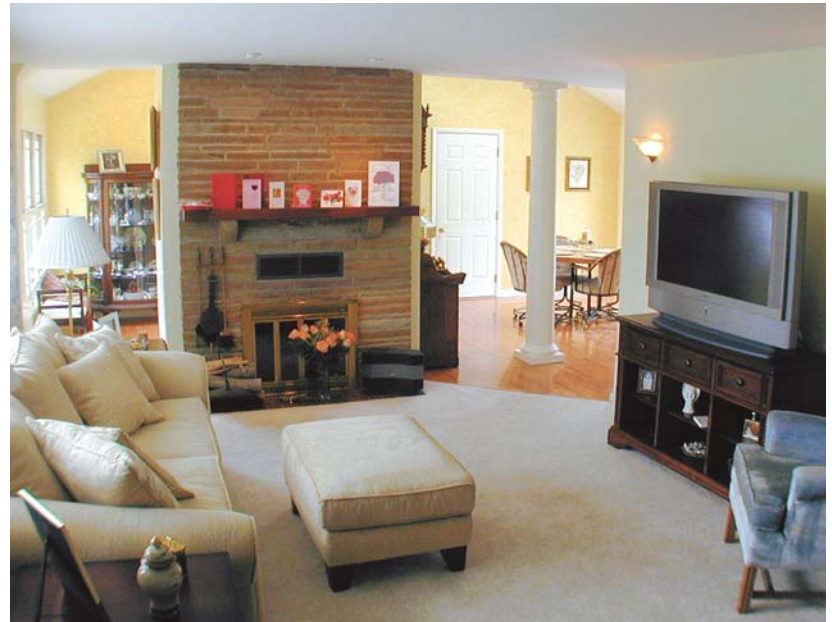
Walls were removed on either side of the fireplace to open up the area.
